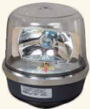
Extra Large Revolving Light Fits 8 ft and 12 ft lighthouses 120v, 35w halogen bulb (13 rpm)
